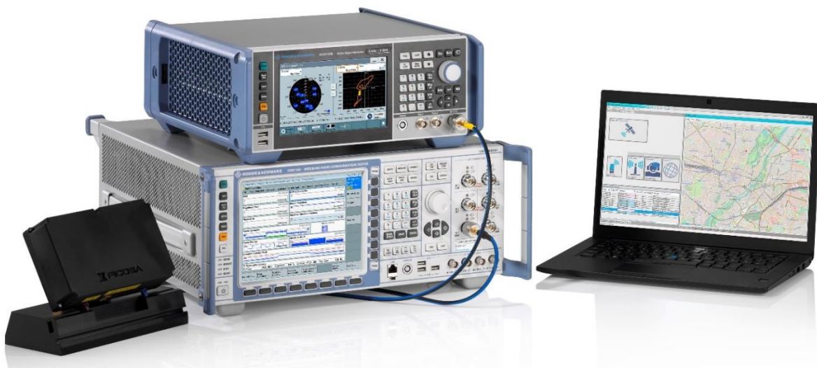
Figure 2: Overview - The test solution with GNSS simulator, wireless radio communication tester and an IVS (DUT)
